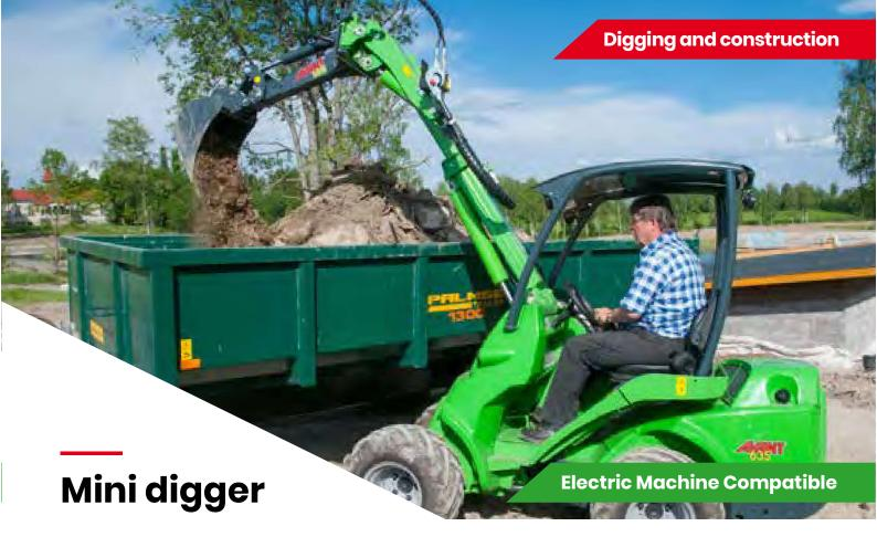
Avant mini digger is an efficient solution for small digging operations where maximum digging depth of 1200 mm or 1500 mm is enough and digging is not an everyday work. It mounts directly on the quick attach plate of the loader and is operated with the auxiliary hydraulics control lever, or with the buttons of the joystick if fitted. Dumping to the side is happens by turning the steering wheel of the Avant.
