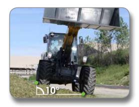
10 DEGREE OSCILLATION Maintain full loads by keeping the tires in contact with uneven terrain.
