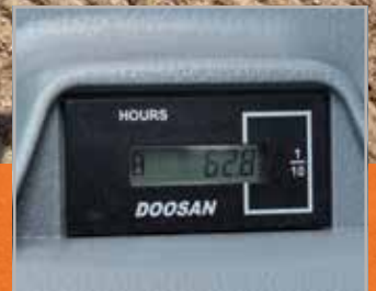
Hour meter (from ground level)
