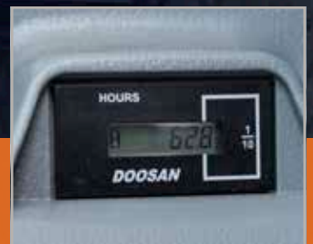
Hour meter (readable from ground level)
