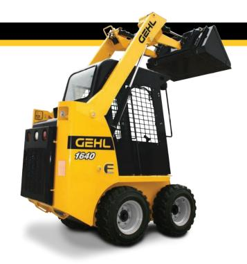
SUPER-COMPACT 36" (909 mm) width with 5.70 x 12 tire option, or 42" (1067 mm) width with 8.70 x 12 heavy-duty flotation standard tires.
