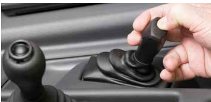
Body hoist lever with boost button
